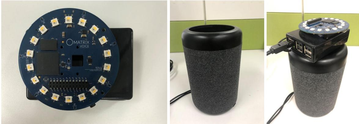
Fig. 1. Left: Raspberry pi 3b with matrix-voice. Center: Omni-directional speaker. Right: System devices together.
